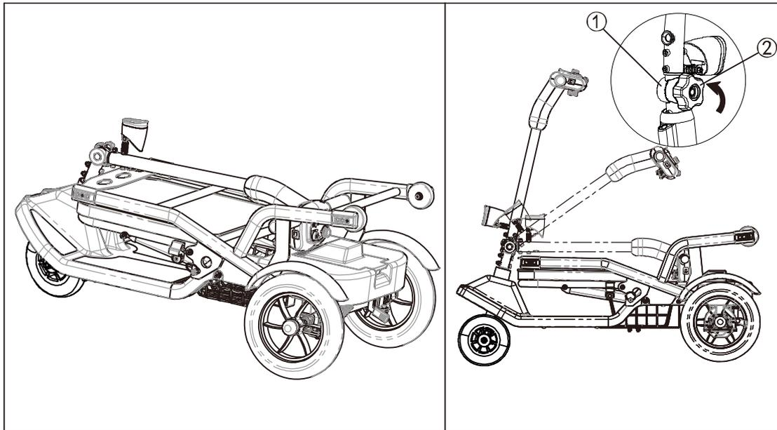
4.1.1.2 Pull the pin(③) out until it comes out of the hole, turn the seat backwards until you hear a "pop", then the pin is automatically locked into the hole, which means that the scooter is fully unfolded. (③ Pin)
